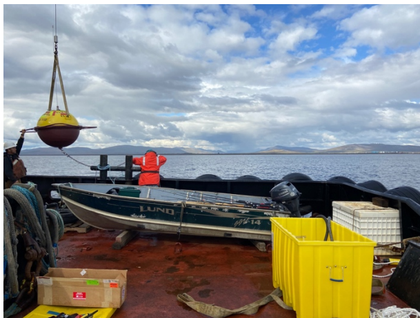
Tug AVIK deployment of the Bering Strait CDIP Buoy off the Port of Nome. Photo Credit: Lucas Stotts, Harbormaster, Nome.
