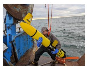
**EAFM Gliders**- UAF successfully completed its first AOOS Ecosystem Approach to Fisheries Management (EAFM) glider sea-trial in the southeastern Bering Sea in July. The primary mission was to assess how well the glider operates in the shallow water and strong tide environment of the region (spoiler: quite well!). A secondary mission was to detect tagged crabs from an ADFG study. CTD and EAFM ecometrics dashboard data from the 19-day June deployment can be found here.
